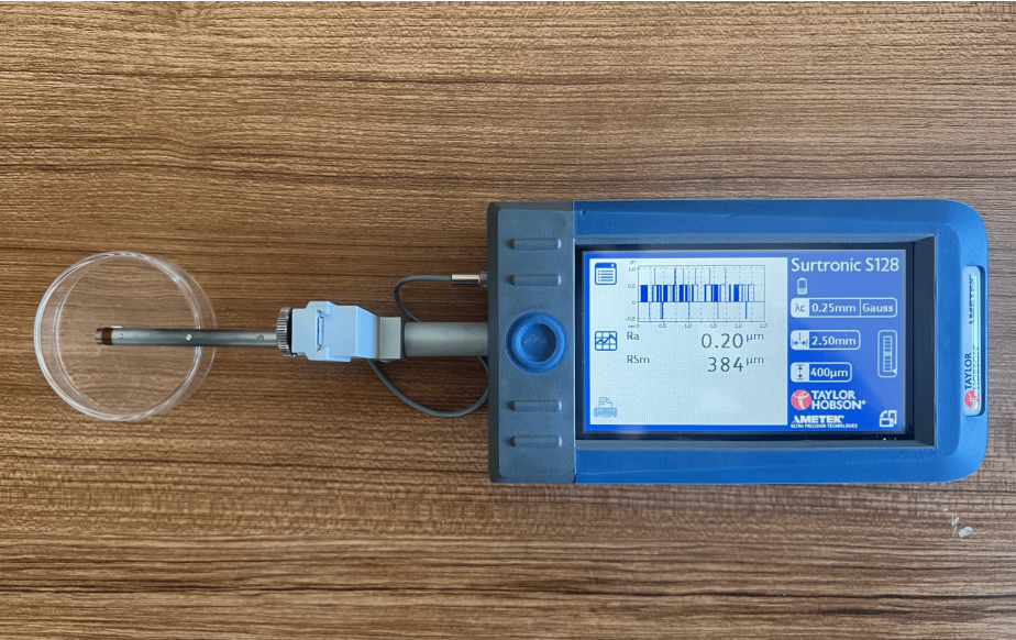
FIGURE 4: Surface roughness measurements performed using a contact profilometer (Surtronic S-100, Taylor Hobson, UK) on restorative material specimens.
